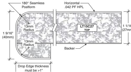
*NOTE: Drop edge not available for 30mm and 40mm windowsill thicknesses.*
