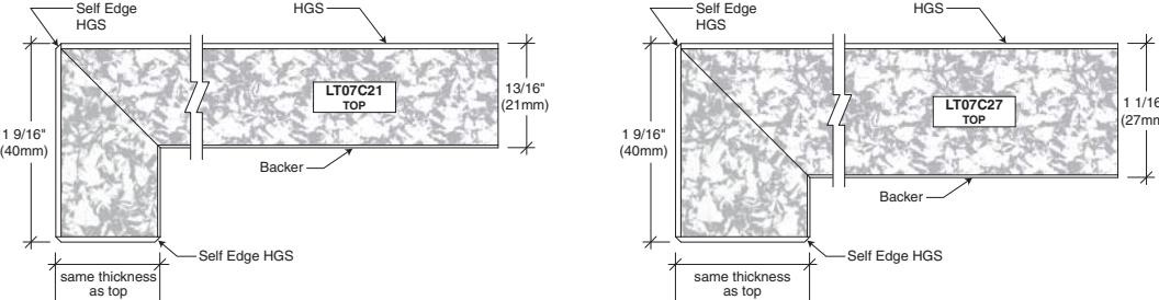
The diagram shows two variations of a windowsill with a drop edge. Both variations feature a "Self Edge HGS" on the left side and a "Backer" layer underneath. The top surface is labeled "HGS" and "LT07C21 TOP" or "LT07C27 TOP". The height of the drop edge is indicated by a vertical dimension: 1 9/16" (40mm) on the left variation and 1 1/16" (27mm) on the right variation. The front edge of the drop edge is also labeled "Self Edge HGS". A note states "same thickness as top" for both variations.
